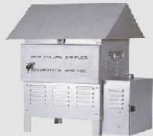
High Volume Sampler APM430 (TSP)
